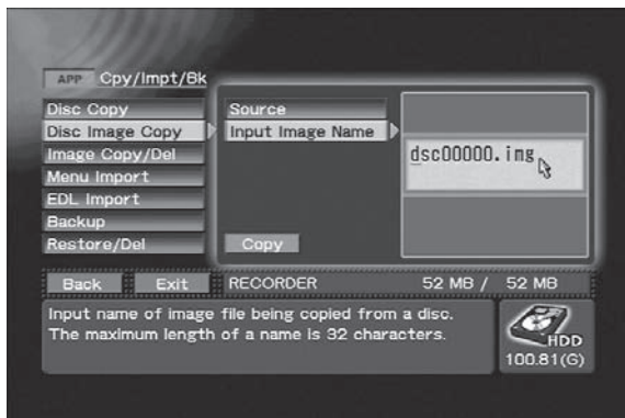
Using APP section → [Cpy/Impt/Bkup] → [Disc Image Copy] → [Input Image Name] to enter a file name
